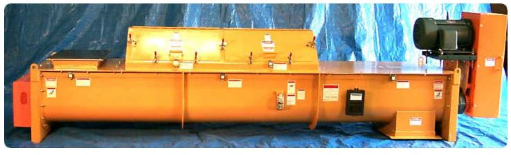
Twin 16" spirals with adjustable reverse pitch mixing paddles in a 14-foot long continuous mixer provide for a rapid and thorough mixing action of liquids to solids. Output is rapid and uniform.
