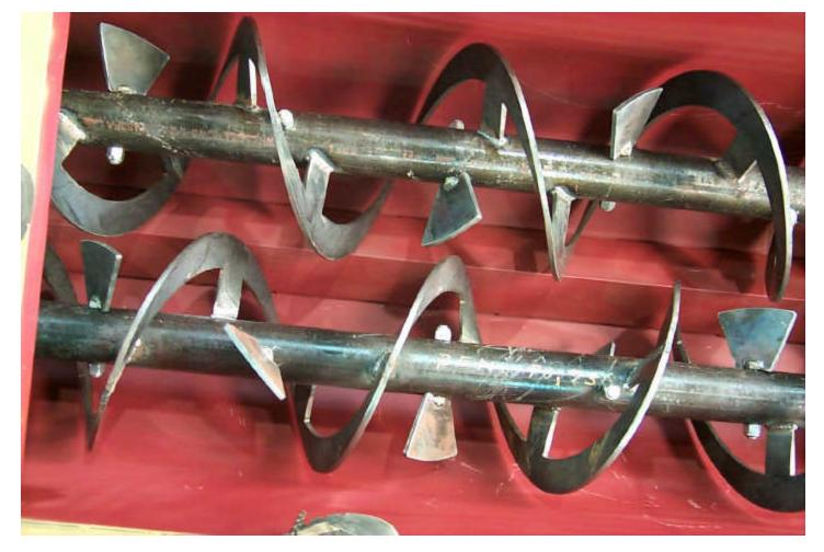
Photo illustrates heavy duty mixing chamber with twin rotor ribbon spirals equipped with adjustable reverse action agitation paddles. This combination of mixing tools provides for an efficient and continuous flow of a uniformly mixed product passing through the mixing chamber.
