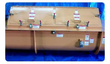
Views above and to the right illustrate the special design of the liquid spray manifold assembly. Note the oversize interlocked hinged inspection and maintenance ports which provide for excellent operator access, machine adjustment and mixed product quality control.
