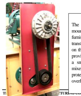
The illustrated 25 HP shaft mounted gear reducer drive is furnished with a hydrokinetic transfluid drive pulley mounted on the motor shaft. This pulley provides for a **"softstart"** and a smooth acceleration of the mixer with continuous protection against operating overloads or stall conditions.
