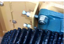
Oversize spiral timing gears and main shaft bearing blocks are examples of heavy-duty construction.
