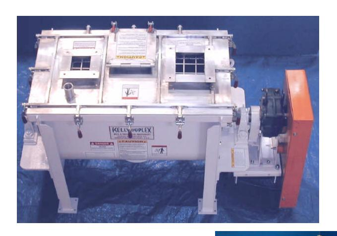
Views illustrate the aluminum top cover, the 3 HP drive and the mixer discharge with no discharge gate for feeding agitated product directly into the downstream extruder.
