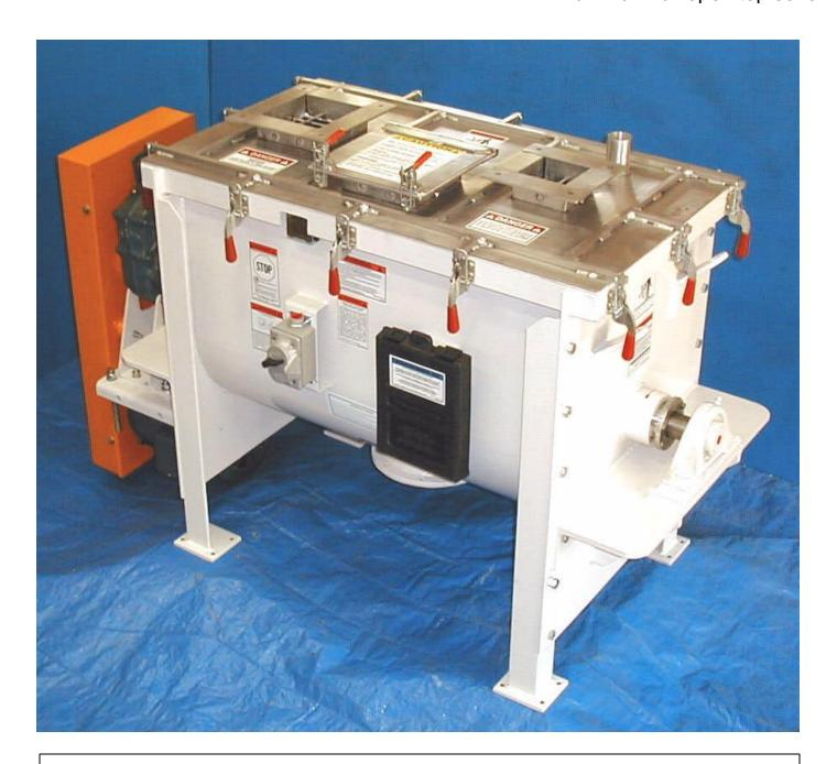
This Model 193 Horizontal shaft paddle mixer is used as an agitated storage reservoir and feeding device to feed plastic pellets and compounds into the inlet of an extruder. Gross vessel capacity is 9 cubic feet. Nominal working capacity is 6 cubic feet. A 3 HP drive turns the mixer's tool arms and mixing tools at 40 RPM. The mixer discharge feeds product directly into the downstream extruder with no intervening discharge gate.
