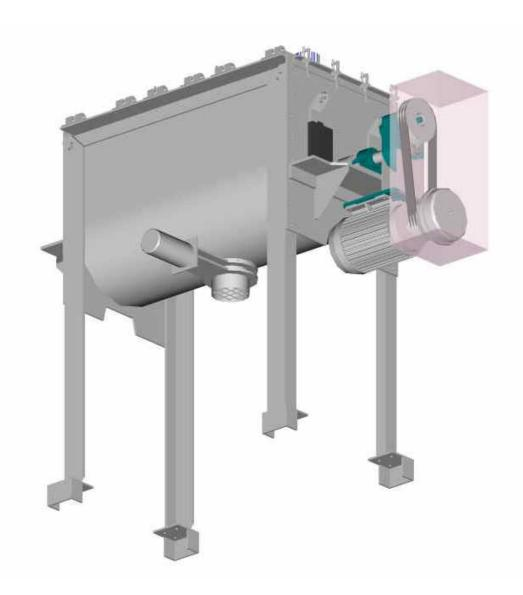
Floor level view of the Model 3206 Mixer reveals the packed air cylinder operated knife gate discharge valve, which provides for a tight mixer and allows for a thorough discharge. The mixer support legs provide for direct discharge into bulk containers, and the leg pads interface directly with an integrated load cell batch weighing system.
