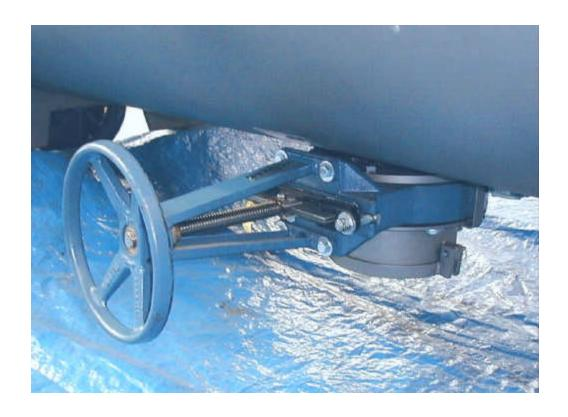
The mixer discharge valve is a packed and sealed knife gate with an extension spout that features a protective grate removable for cleaning and interlocked for operator protection.
