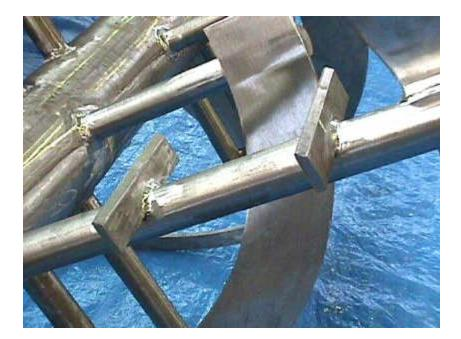
These views show the installation of optional cutters which serve to add an extra measure of agitation to the mixing action of the ribbon assembly.
