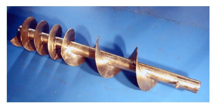
Views of the spiral above illustrate stepped pitch T304SS flighting continuously welded to T304SS pipe and polished. Drive and tail ends are slotted to provide slip together disassembly for frequent cleaning.
