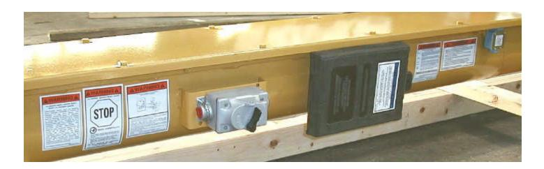
View illustrates conveyor standard accessories: Padlockable Protective Interlocking Electrical Control Switch (PCS), Protective Interlocking Limit Switch (PLS), Operator's Manual Case (OMC), and instruction and hazard warning decals.
