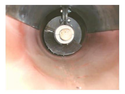
Exterior and interior views illustrate a shroud mounted inside the conveyor U-trough and an intermediate hanger bearing
