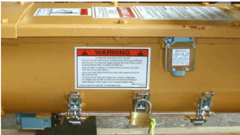
Hinged trough inspection panel with PLS
