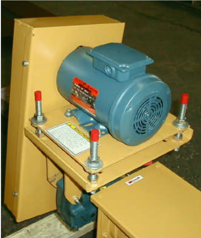
2 HP SMGR Drive at 100 RPM
