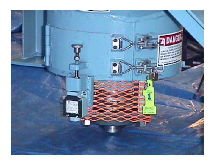
Time Delay Protective Interlocking Limit Switch
