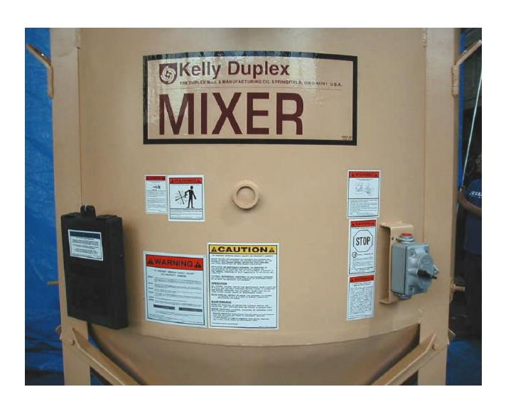
Standard mixer equipment includes an Operator's Manual Case, a Padlockable Interlocking Electrical Control Switch and hazard warning and instructional decals. These items are illustrated above.
