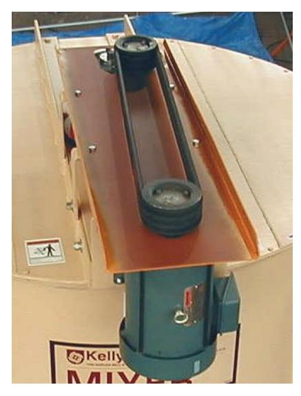
The 5 HP shaft mounted gear reducer and v-belt drive is mounted on top of the vertical mixer. This durable, compact, and easily serviced drive takes both the end thrust and radial load of the mixer spiral.
