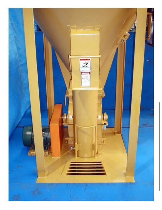
The view at left shows the hammermill drive and the mixer inlet hopper at floor level for addition of feed ingredients. Also shown is the bagger discharge at 34" discharge height. Installation is simple and the floor space required is only 20 square feet. The height of the mixer above the floor is 8-1/2 feet.
