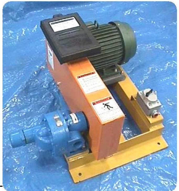
5 HP molasses/fat pump with adjustable built in by-pass valve. Complete with motor and drive. 250 pounds
